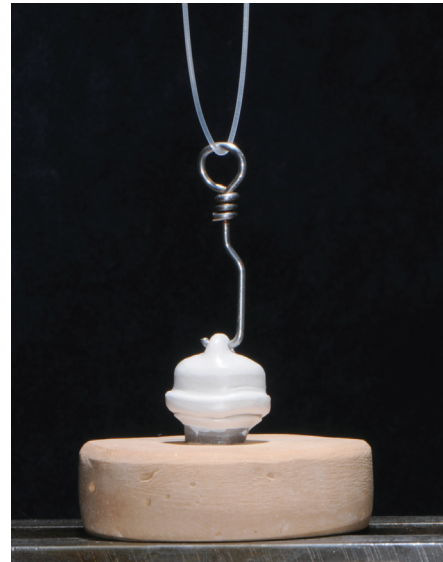
Fig. 5 Specimen positioned in a Universal Testing Machine, chain clipped on secondary crown clamp.
