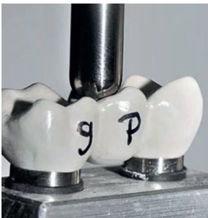
Fig. 19: BioHPP bridge during the test. 24)
