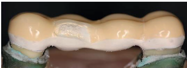
Fig. 39: Bridge after load test with chipped veneer. 52)
